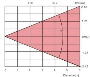
The Projector is best to be placed 5 meters from wall, and from this distance the light effect will cover an area of 4 m x 4 m.
